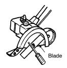
To remove the blade, insert a screwdriver into the hole in the gearbox; then, remove the nut (clockwise), washer and blade from the blade shaft.
